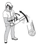
If the kickback is less violent or the kickback zone of the bar is closer to you the chain brake is designed to be activated manually by the movement of your left hand.
